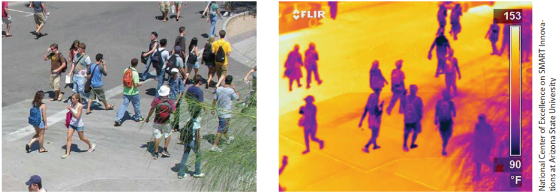
Figure 41: Conventional pavement temperatures during summer. Temperature reaches up to 67°C (EPA, 2012)
