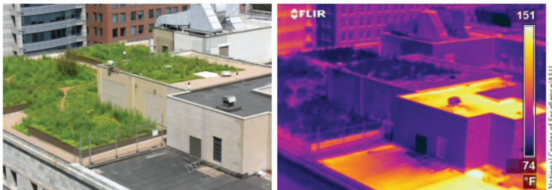
Figure 40: Temperature differences between a Green and Conventional Roof. Green roof is almost 40 °C cooler than the neighboring conventional roof
