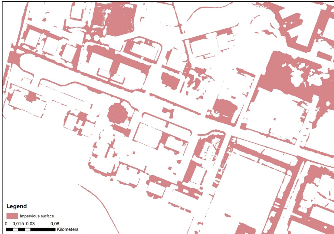
Figure 4-4: Impervious surfaces - Detail at building scale
